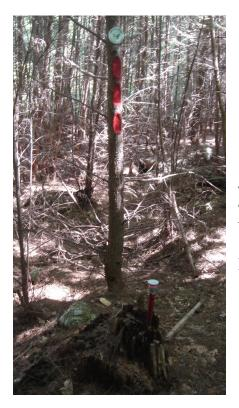
"BB" is a rebar set in a stump with an aluminum cap marked "Meridian Land Services, Inc." located westerly of a triple blazed Hemlock with a HCC marker as witness.
