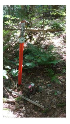
"DD" is a rebar with aluminum cap marked "Meridian Land Services, Inc." located west of an orange fiberglass post with a HCC marker as witness.
