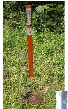
"J" is a ½" diameter rebar with a red plastic cap marked "PD MELLEN LLS 815" located 1.2' east of an orange fiberglass post with HCC marker as witness. It is located just slightly west of the centerline of the Hillsborough S&W Commission sewer easement.
