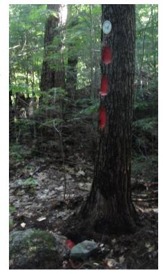
"F" is a drill hole in a boulder, with an orange fiberglass post with HCC marker as witness.
